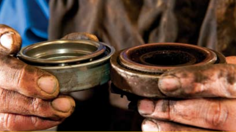
Here you can see the hot spots, a result of excess clutch slipping
