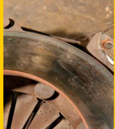
Grooves cut into the diaphragm spring by the release bearing, a result of resting the foot on the clutch pedal
