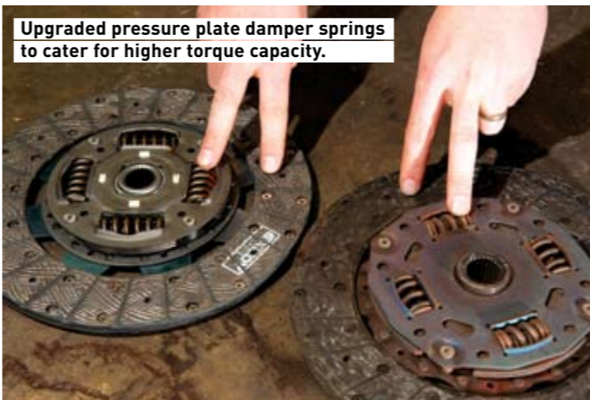
Premium friction materials on the disc increase clutch durability and burst strength
